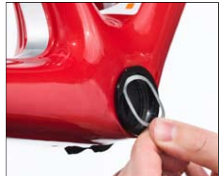
Figure 44. Inserting the Wave washer (after the washer) on the non-drive side
